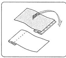
There are two blind hem stitches on your machine. The regular blind hem is used for woven fabrics. The stretch blind hem is wider and will "give" and is used for knit and stretch fabrics.
